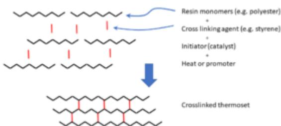
Illustration of the molecular crosslink formation for a thermoset polymer.
