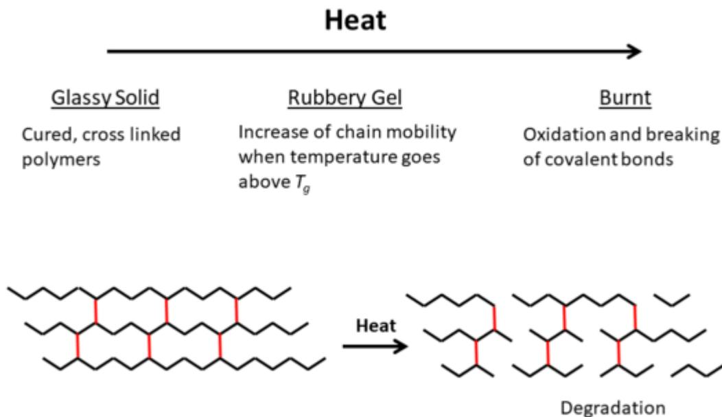
Thermoset polymer breakdown if subjected to high thermal breakdown temperatures.
