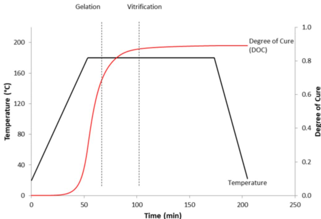
Example of a thermoset polymer heated cure cycle process showing the crosslink development (degree of cure). .
