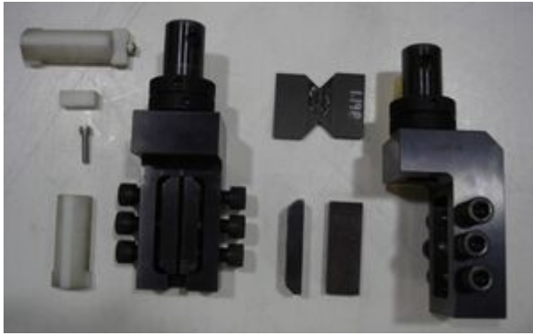
ASTM D7078 V-Notched Rail shear test fixture.
