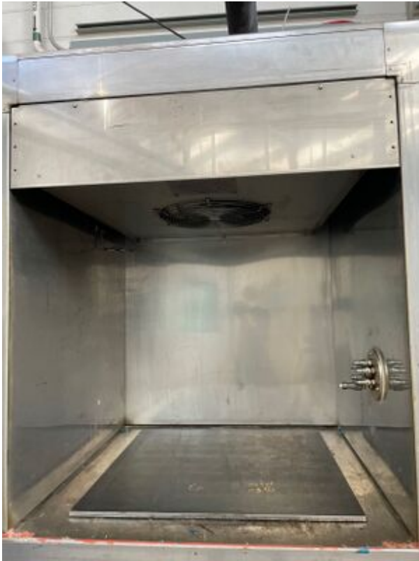
Oven with air being blown top down
