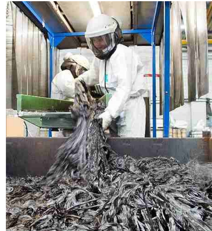
Char residue from polymer decomposition
