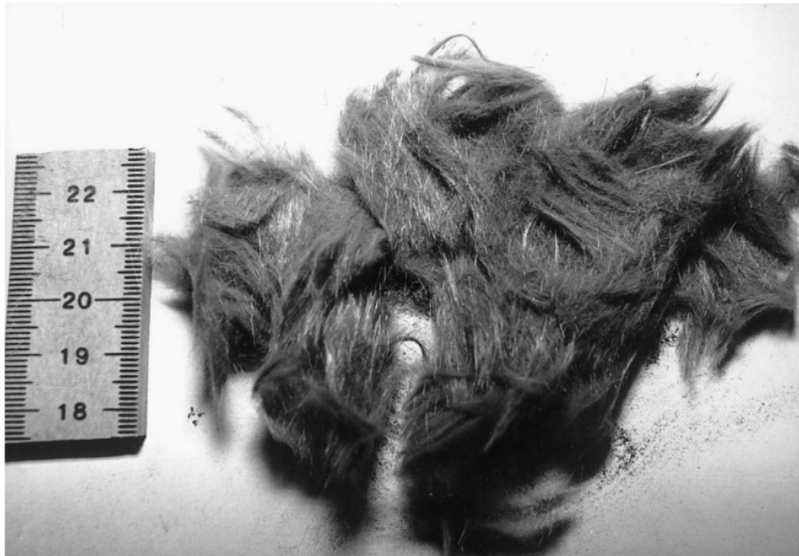
Fig. 7. Fibre product recovered from SMC feed.
