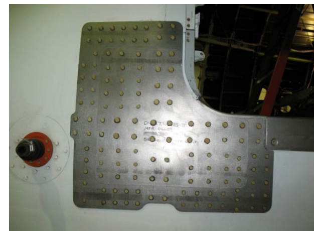
Bolted repair on an aircraft [2]
