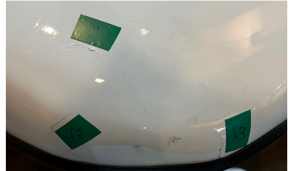
BVID can appear as small cracks on the surface (courtesy of UBC Supermileage)
