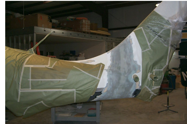
Bonded repair of aft fuselage skin of a small aircraft [1]
