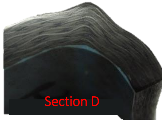
Wrinkling in a textile carbon fiber laminate
