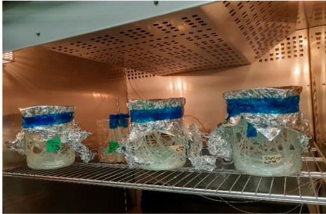
Aging oven / immersion beakers
