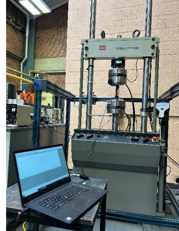
Universal testing machine with AE monitoring
