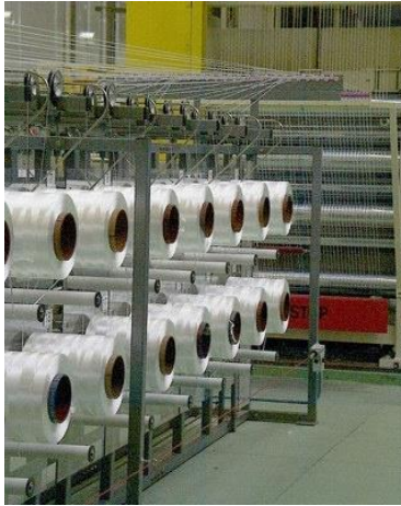
Precursor Unwinding Creel (Courtesy of Texkimp Ltd.)
