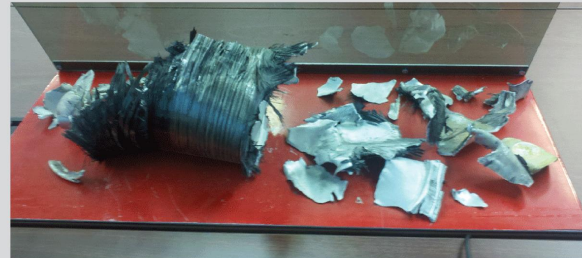
Filament Wound Tank After Burst Test
