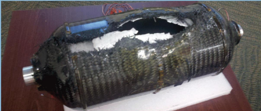
Braided Tank After Burst Test
