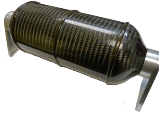
Filament Wound Tank After Burst Test
