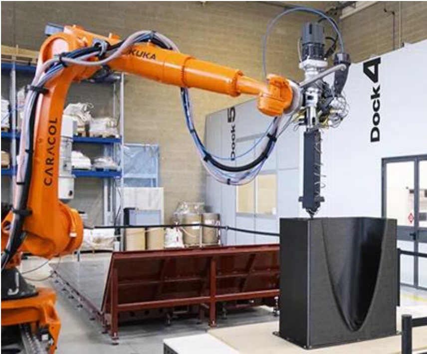
AM of a composite autoclave mold for carbon fiber lamination of a drone nose structure [1]
