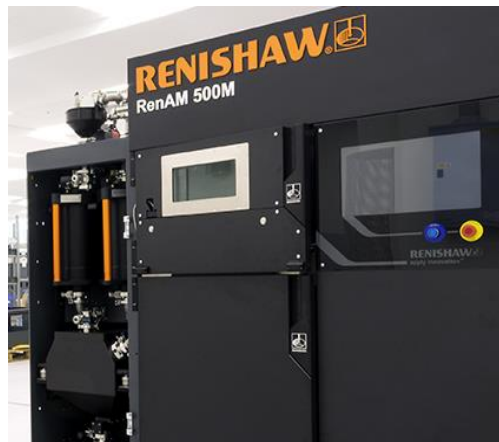
Industrial-scale AM for metals (Renishaw 500M)
