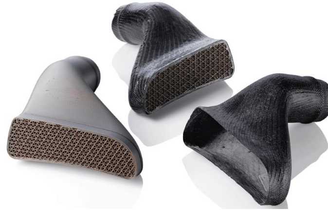
Photo of hollow complex part with sacrificial interior support using a thermoplastic material dissolvable in a basic solution [2]
