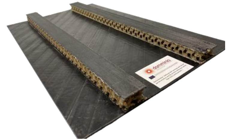
Photo of a demonstrator composed of CF/LMPAEEK laminate produced by AFP and a composite core by FFF printing of PEKK filament [3]
