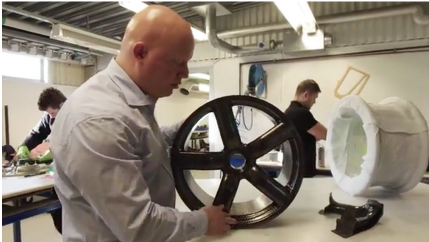
Koenigsegg wheel made with prepreg/autoclave
