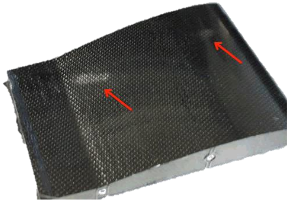
Dry spots (voids)
