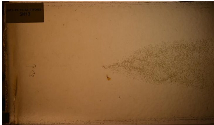
Porosity caused by pin-hole in vacuum bag
