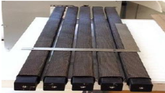
Basic preforms assembled over mandrels
