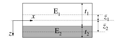
$$A = \sum_{k=1}^{n} E_k \cdot t_k \qquad \qquad \overline{z}_1 = -\left(\frac{t_1 + t_2}{2} - \frac{t_1}{2}\right) = -\frac{t_2}{2}$$
