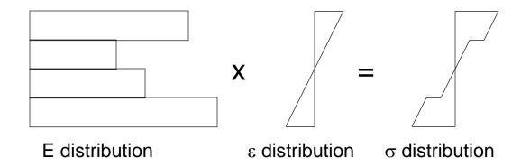
Note that the linear strain distribution relies on the assumption that there is perfect bonding between the layers
