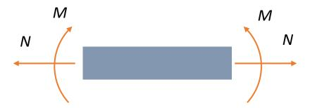
• Two types of deformation are considered for a laminated beam: mid-plane axial strain and curvature:
