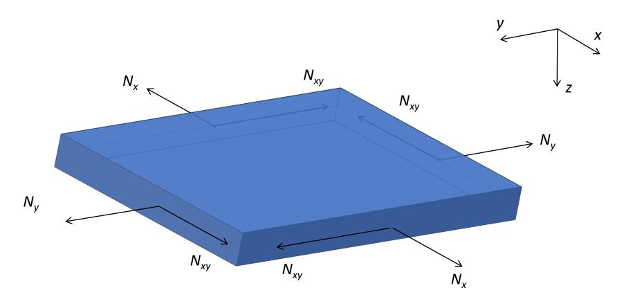
Through thickness forces  $(N_z, N_{zx} \text{ and } N_{yz})$  are ignored for a thin plate
